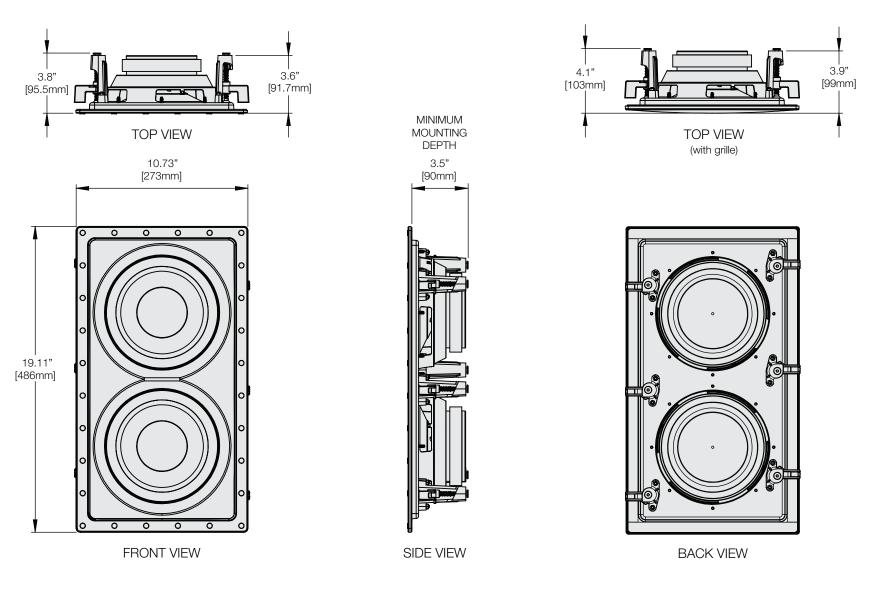
OVERALL DIMENSIONS: (H) 19.11" [486mm] x (W) 10.73" [273mm] x (D) 4.1" [103mm] WEIGHT: 26.2lbs (11.9kg) each
